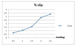
Fig. 12: Slip Vs Load
