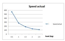
Fig. 11: Speed Vs Load
