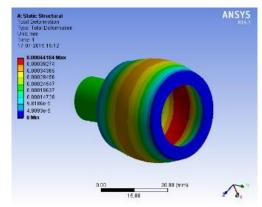
Fig. 6: Total Deformation of Thruster Body
